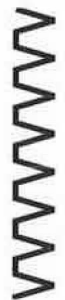
7 Vari-overlock Specially for fine synthetic and silk jerseys, Helanca and fine cotton and wool jerseys
